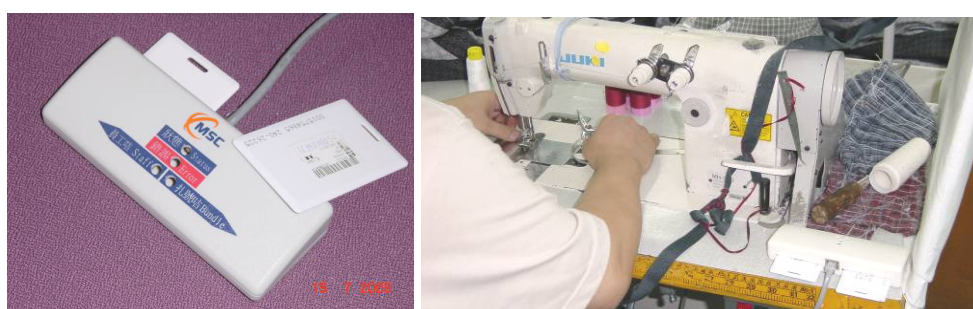
Photos: MSC's R&D Department will create the setup for running the RFID on the site. There will be a low-cost tag smart card and reader next to each of the sewing machines for recording the details of work by each staff.
