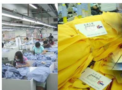
Photos: The traditional use of paper-based work record, compared with MSC's RFID record card during the WIP process flows. The traditional method looks set to be replaced.
